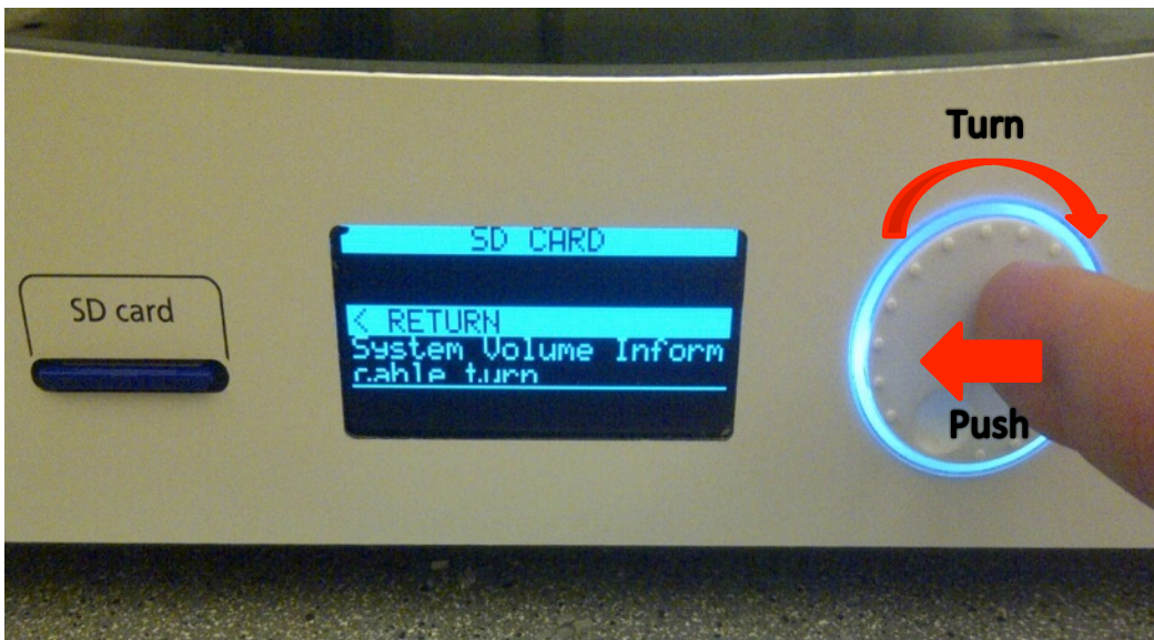
Step 18: Scroll through the files by turning the wheel, to find the desired file to be printed, and select the file by pushing the wheel. DONE! The printer will begin automatically.
